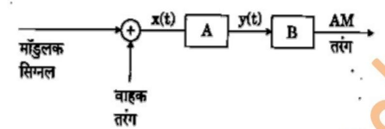
In the block diagram of a simple modulator for obtaining an AM signal, shown in the figure, identify the boxes A and B. Write their functions.
