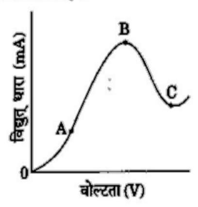
The graph shown in the figure represents a plot of current versus voltage for a given semiconductor. Identify the region, if any, over which the semiconductor has a negative resistance.
