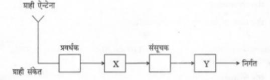
In the given block diagram of a receiver, identify the boxes labelled as X and Y and write their functions.
