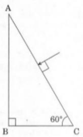
Trace the path of a ray of light passing through a glass prism (ABC) as shown in the figure. If the refractive index of glass is  $\sqrt{3}$ , find out the value of the angle of emergence from the prism.
