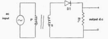
As shown in the figure above the a.c input is applied across the primary of transformer. The secondary is connected to junction diode and load resistance (Rc) in series.
