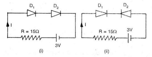
In circuit (i) Both D1 and D2 are forward baiased hence both will conduct current and resistance of each diode is "0". Therefore I = 3/15 = 0.2 A (ii) Diode D1 is forward bias and D2 is reverse bias, therefore resistance D1 is "0" and resistance D2 is infinite. Hence D1 will conduct and D2 do not conduct . No current flows in the circuit.
