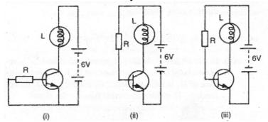
In fir (i) emitter –base junction has no source of emf. Therefore Ic =0, bulb will not glow. In figure (ii) emitter – base junction is forward biased, therefore lamp "L" will glow.
