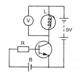
In the given circuit emitter –base junction of N-P-N transistor is forward biased , with battery "B". When "r" decreases  $I_{\rm E}$  increases . Because
